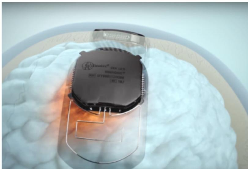
detects the electrical activity in the motor cortex with “minimally-invasive implantation in the cranium and, over the long term, to measure ElectroCorticoGrams thanks to an array of electrodes in contact with the dura mater.”
