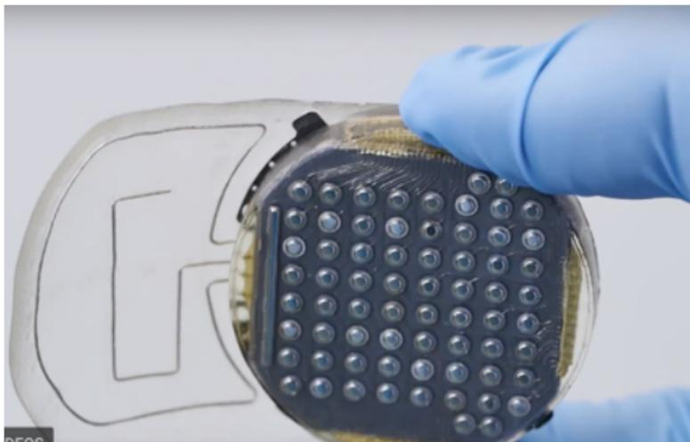
records ElectroCorticoGrams, has remote power supply, and wireless data transfer system.
