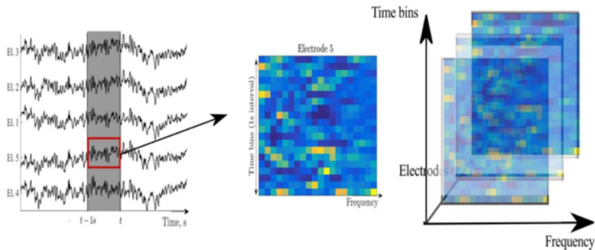
For each electrode a one-second long historical interval  $[t_m - \Delta t, t_m]$  undergoes wavelet transformation and thus obtains feature description in spectral-temporal domain. Merging spectral-temporal feature matrices for all electrodes, one obtains 3D feature description  $X_m$  for the time point  $t_m$ .
